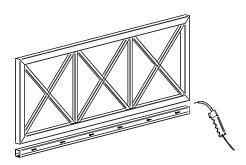
1. Prepare a guide with lenght Sand weld it under the gate.
