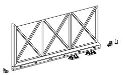
3) Slide the gate guide over the trolleys and fix the Guide Roller on one end and a Guide Roller and/or the Front Cover on the other end.
